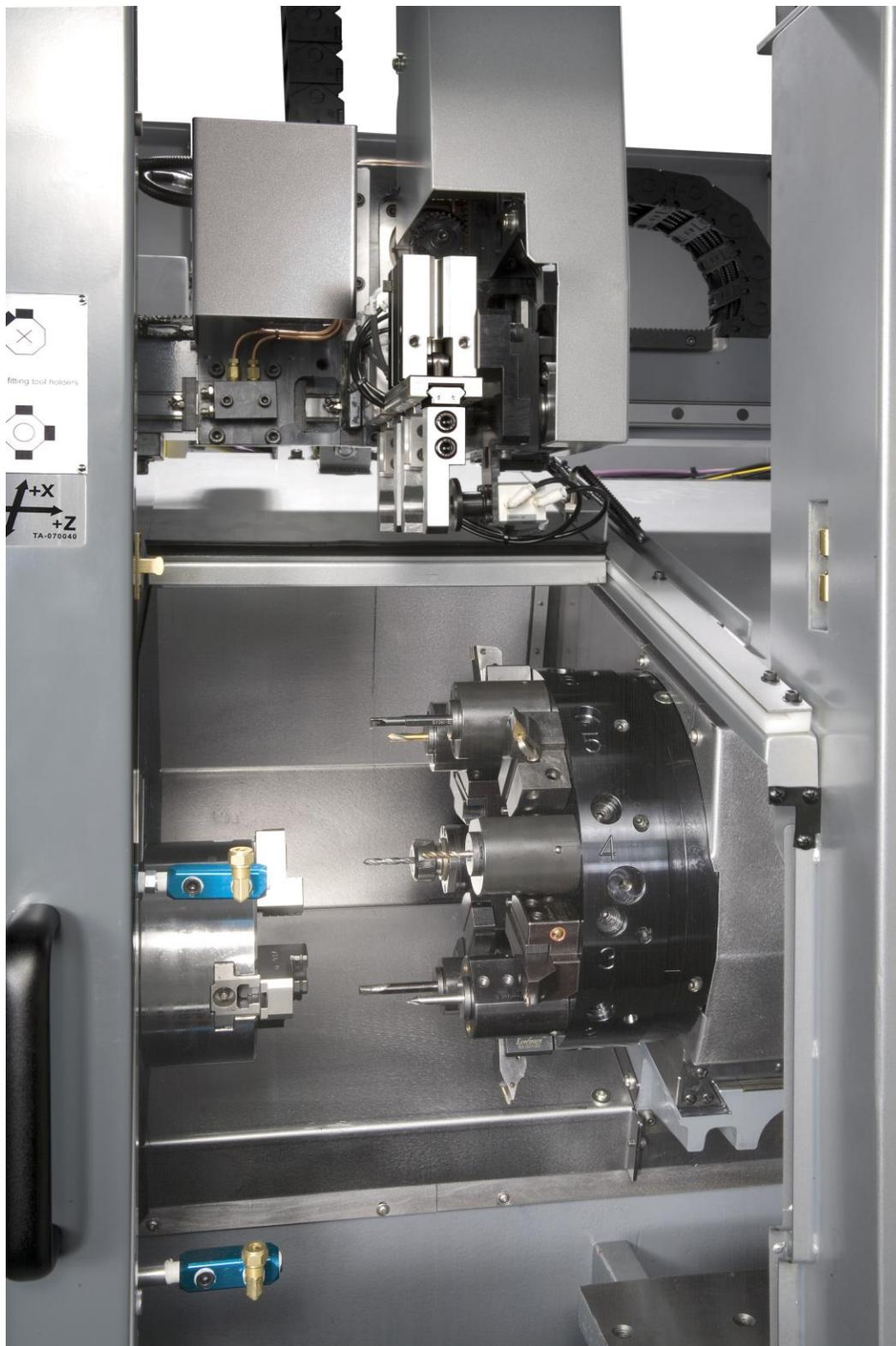
Optional VDI-30 (or BMT-55) Driven Tools Turret pictured above. Bolt on tooling is standard.
